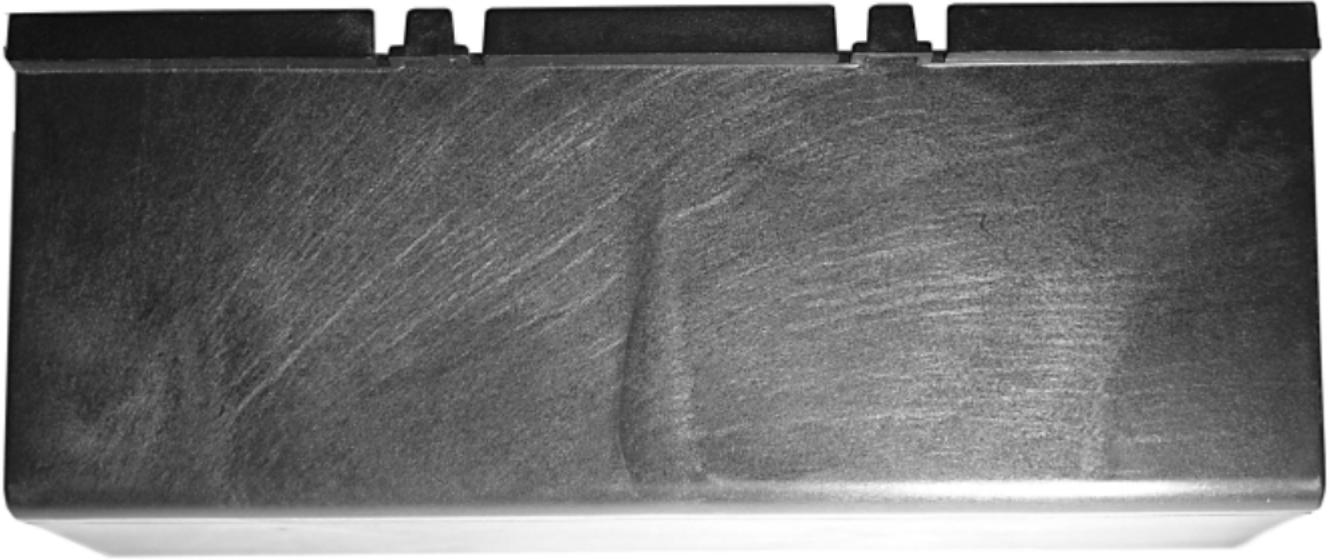
Figure C.8: Picture of one part side (in this rear view, the injection gate is on the left)
